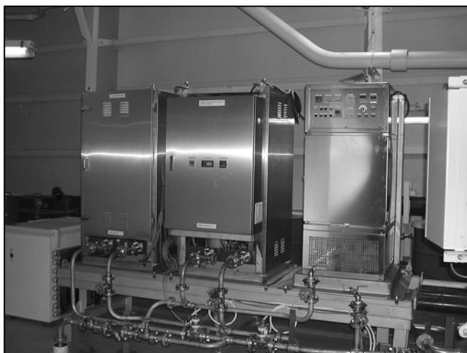
Figure 1 Photograph of marine pollution observation system on board the bulk carrier.
